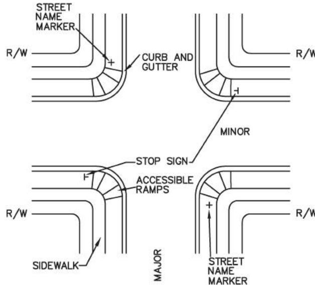
INTERSECTION with CURB and GUTTER
