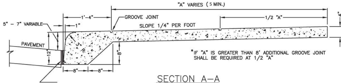
TWO 1/2" THICK PIECES BITUMINOUS FIBER REQUIRED IF SUBBASE IS CONCRETE. MUST BE SEALED WITH APPROVED JOINT SEALER.
