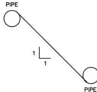
THE SANITARY SEWER AND STORM DRAINAGE PIPES MUST BE NO CLOSER TOGETHER HORIZONTALLY THAN THE VERTICAL DISTANCE BETWEEN THE TOP OF THE HIGHER PIPE AND THE BOTTOM OF THE LOWER PIPE. A MAINTENANCE CREW MUST BE ABLE TO DIG DOWN TO THE LOWER PIPE SLOPING THE DITCH ON A 1:1 SLOPE AND NOT EXPOSE THE HIGHER PIPE.
