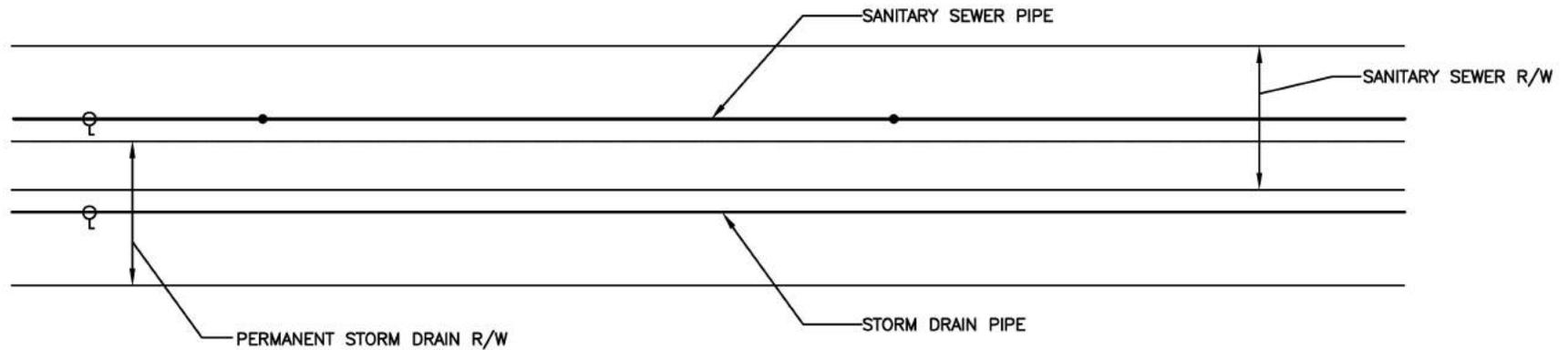
THE SANITARY SEWER AND STORM DRAINAGE RIGHTS OF WAY MAY OVERLAP; HOWEVER THE PIPE AND ASSOCIATED STRUCTURES MUST NOT BE IN THE OTHER UTILITY'S RIGHT OF WAY. THE SANITARY SEWER RIGHT OF WAY WIDTHS SHALL BE AS OUTLINED IN C.M.U.D.'S DESIGN MANUAL. THIS DETAIL DOES NOT APPLY TO STORM DRAINAGE UTILIZING OPEN CHANNEL FLOW.
