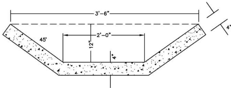
SLOPE DRAIN, BASE DITCH OR BERM DRAINAGE
